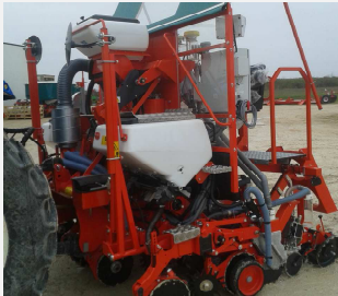
Volumetric fertilizer with discs Hydraulic assistance to fold the liner
