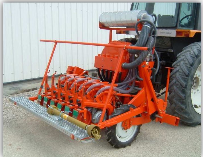
Semi-automatic “stop at plot” version with electric valve and gear motor
