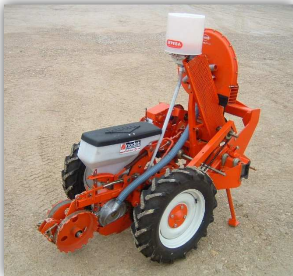
Semi-automatic “stop at plot” version with electric valve and gear motor
