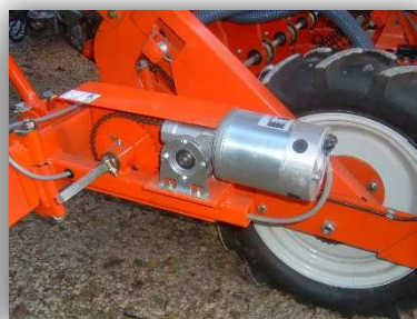
Semi-automatic “stop at plot” version with electric valve and gear motor
