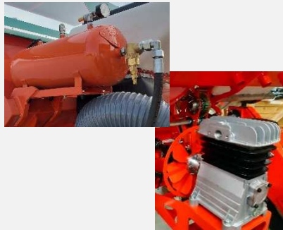
Compressor Pressure gauge controller
