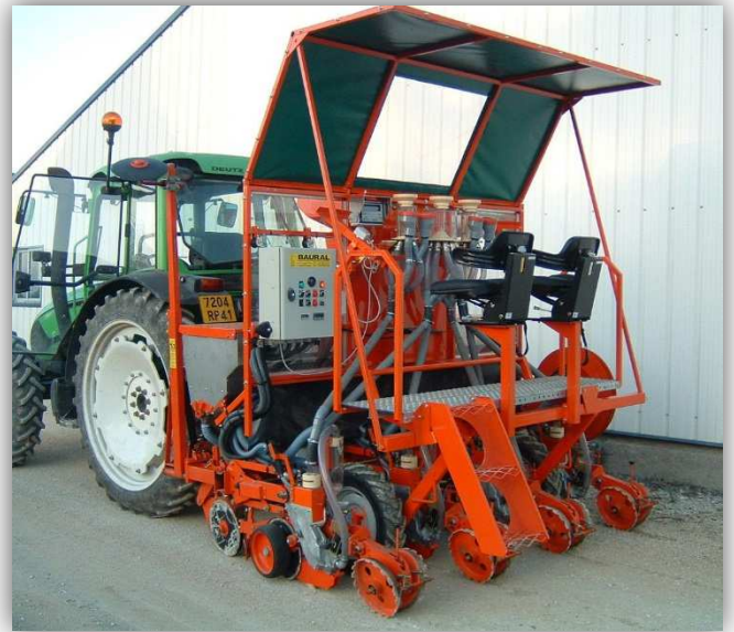
Continuous « non-stop » version with manual cycle start by cable on winder
