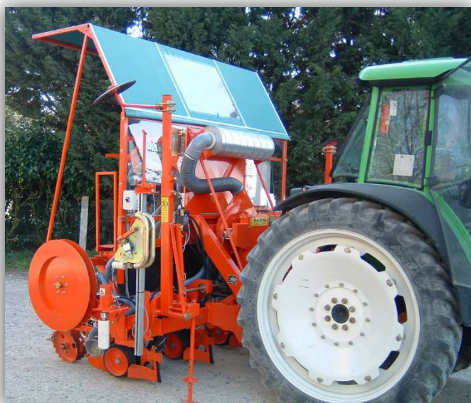
Continuous « non-stop » version with manual cycle start by cable on winder
