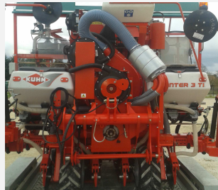
« Insecticide, herbicide, anti-slug » pneumatic microgranulator Turbine with muffler
