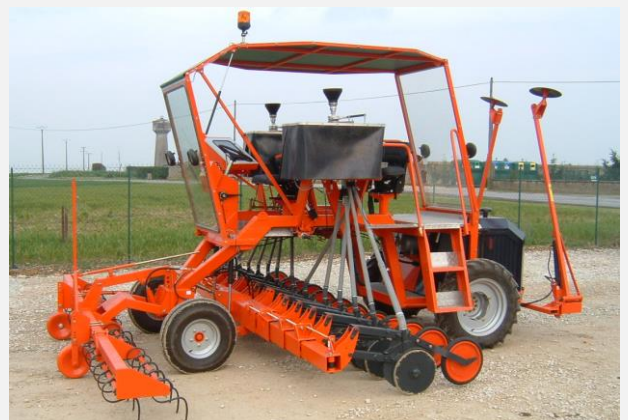
Telescopic girder Seeding with double KUHN discs
