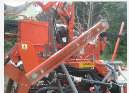
Fertilisor and telescopic girder from 45 to 80 cm
