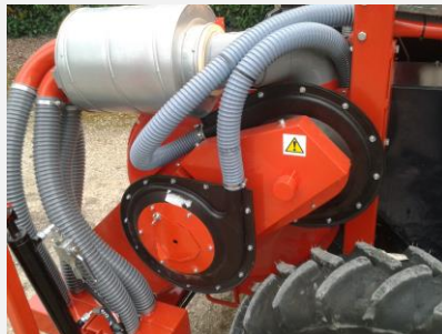
Double turbine for pneumatic transport
