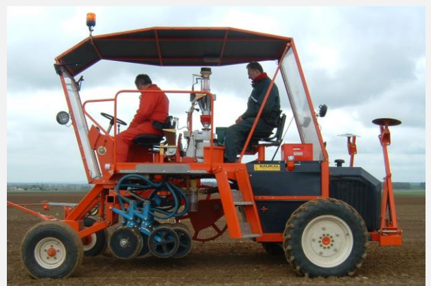
Seeding with double LEMKEN discs Pneumatic transport of seeds
