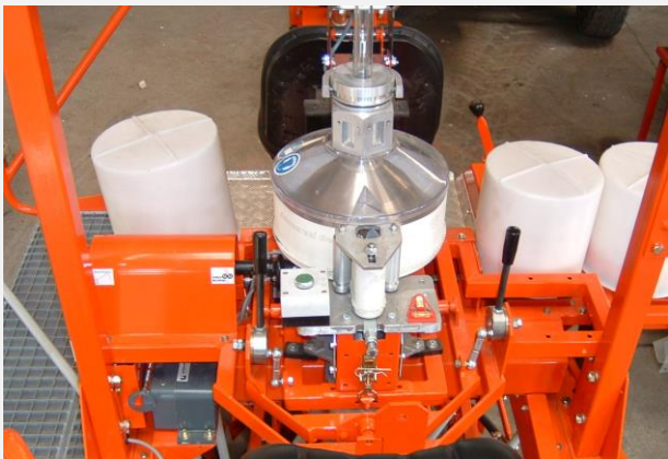
Distribution head with manual or automatic leveling
