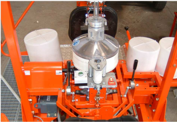
Distribution head with manual or automatic leveling
