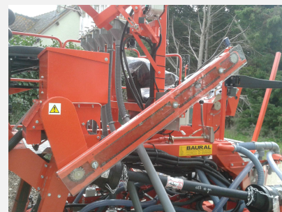
Fertilisor and telescopic girder from 45 to 80 cm
