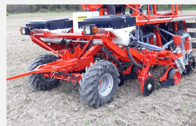
Fertilisor and telescopic girder from 45 to 80 cm
