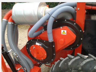
Double turbine for pneumatic transport
