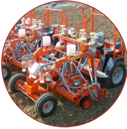
Distribution head with manual or automatic leveling
