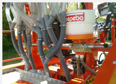
Mechanical Sepeba micro-granulator
