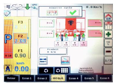
Seeder state and settings are displayed on your ISObus tablet in your tractor or directly on the seeder Increased seeding speed and shorter alleys with the disk acceleration You have all the seeder informations, settings and controls Density, alleys lenght and GPS signal offset can be adjusted easily Or adjust your density automatically with the dose modulation Manual control on the hatchs, divisor and motors
